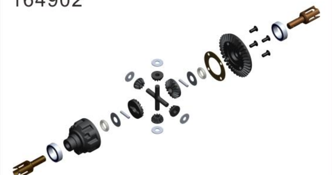
GEAR DIFFERENTIAL FOR 35T - SET
